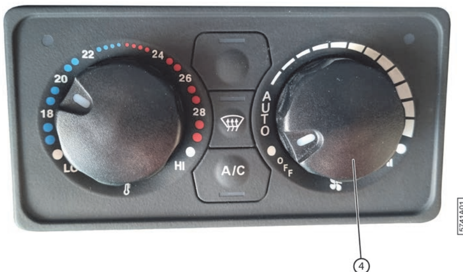
Fig. 95: Switching OFF the climatisation
