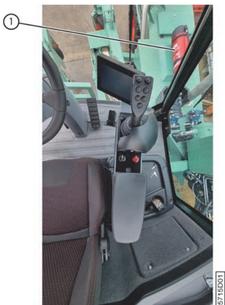
Fig. 38: Location of the fire extinguisher
