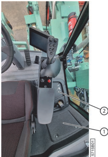
Fig. 32: The electrical cabinets in the cabin
