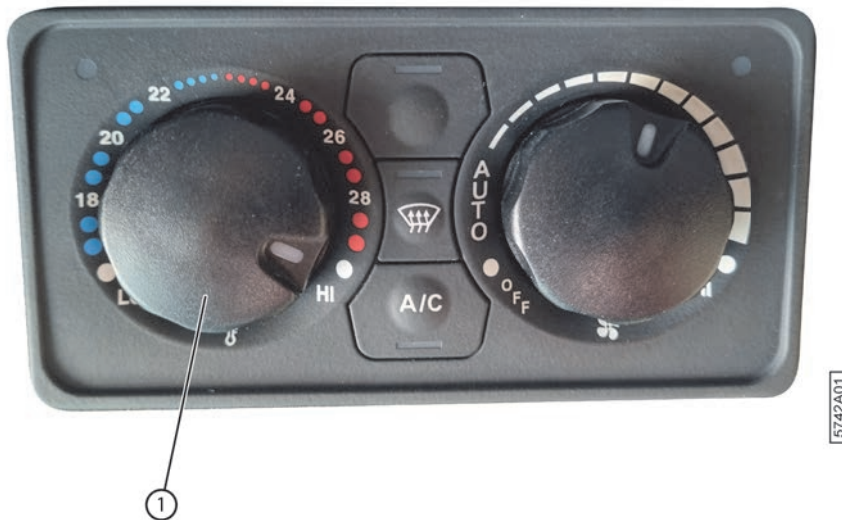
Fig. 96: Switching ON the heating
