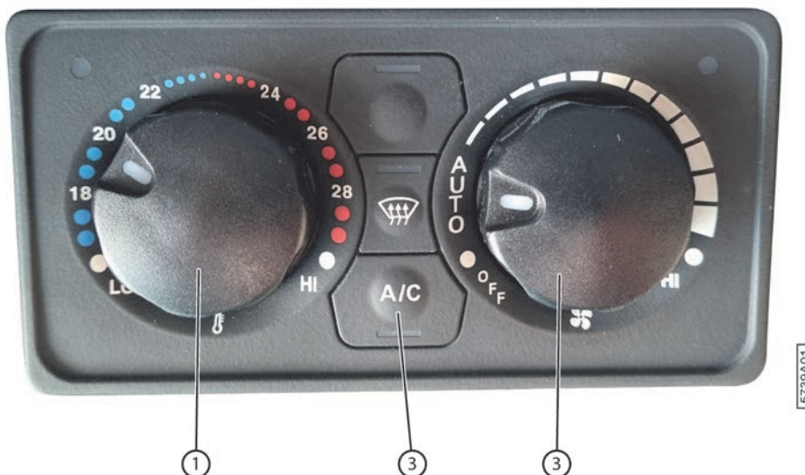
Fig. 93: Placing the air conditioning system in automatic mode
