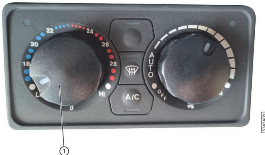
Fig. 97: Switching ON the cooling
