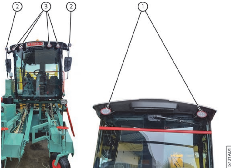
Fig. 15: The work lights
