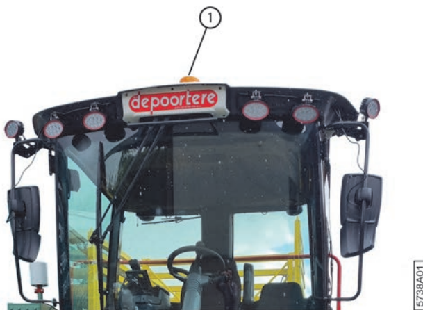
Fig. 13: The flashing light
