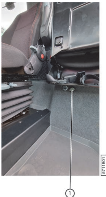
Fig. 30: The 12-volt connection
