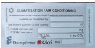
Fig. 125: The sticker with information about the air conditioning
